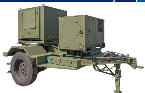
The ZeroBase® EMPAC-T™ 10kW Hybrid Power System (HPS) is a ruggedized military trailer system capable of providing clean, wellregulated power while increasing the efficiency of power generators, supplying backup power in the event of a loss of generator availability, and providing extended silent operations. The 10kW trailered HPS is designed to meet MIL-STD 810G environmental and mechanical specifications to support use in extremely harsh environments across the globe.
